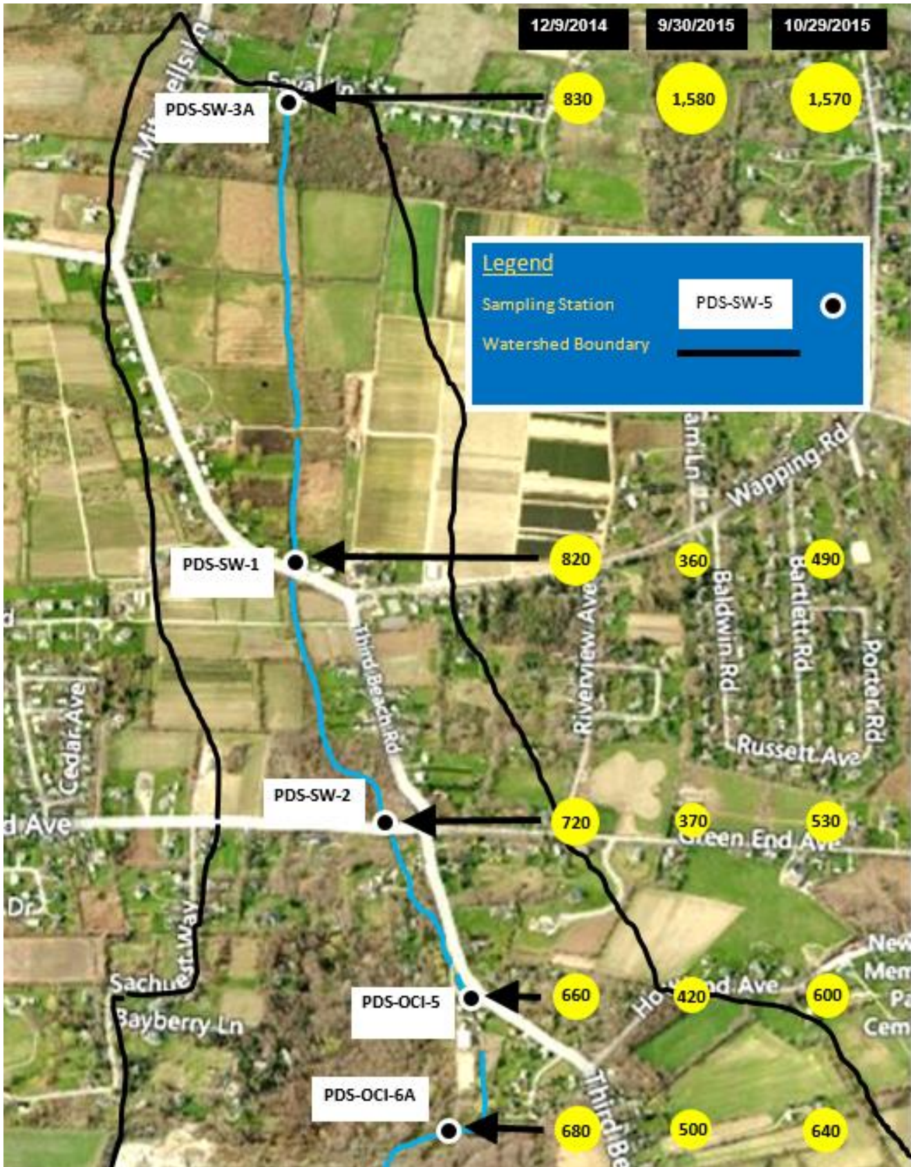
Figure P12. Paradise Brook Wet Weather Nitrate (ug/l).
