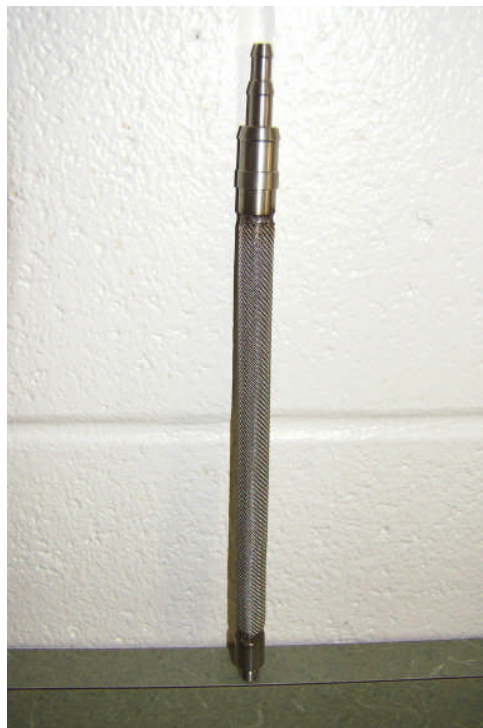
Photo 32: View of typical stainless steel sub-slab sampling probe.
