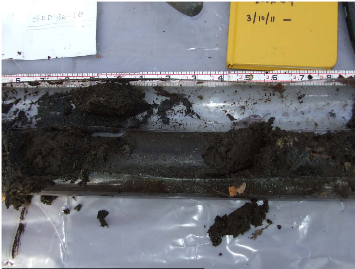
Figure 4.6 - Sediment Core SED 36 – Outer Cove in Channel Sample Interval 1-8 feet December 2011 Sediment Sampling Program
