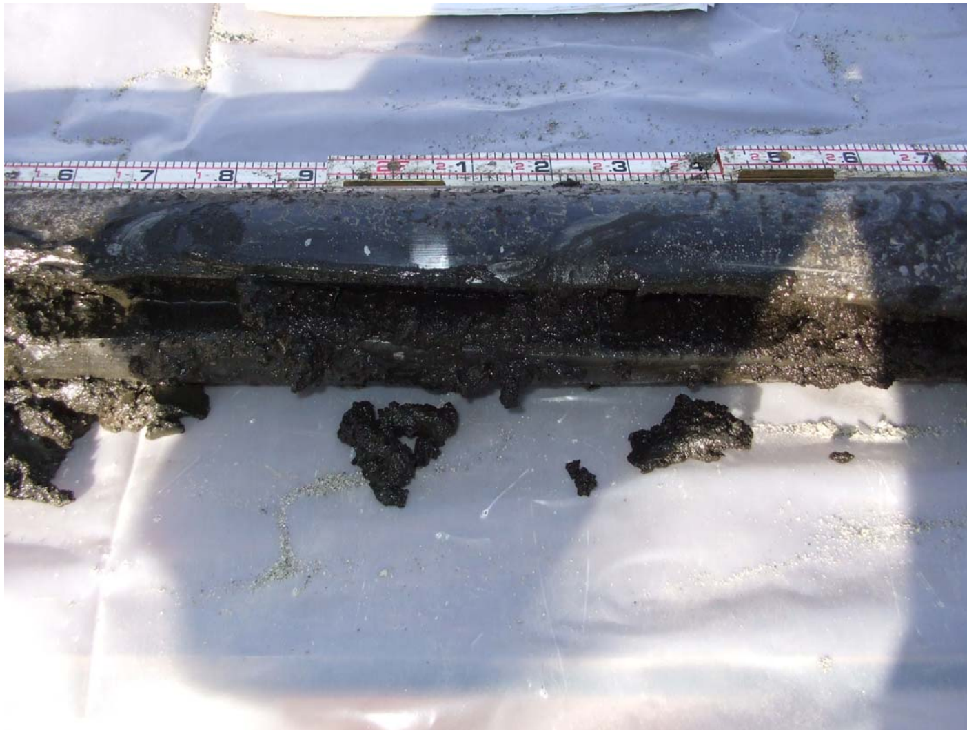
Figure 4.8 - Sediment Core SED52 - Mashapaug Pond Sample Interval 1-4 feet December 2011 Sediment Sampling Program
