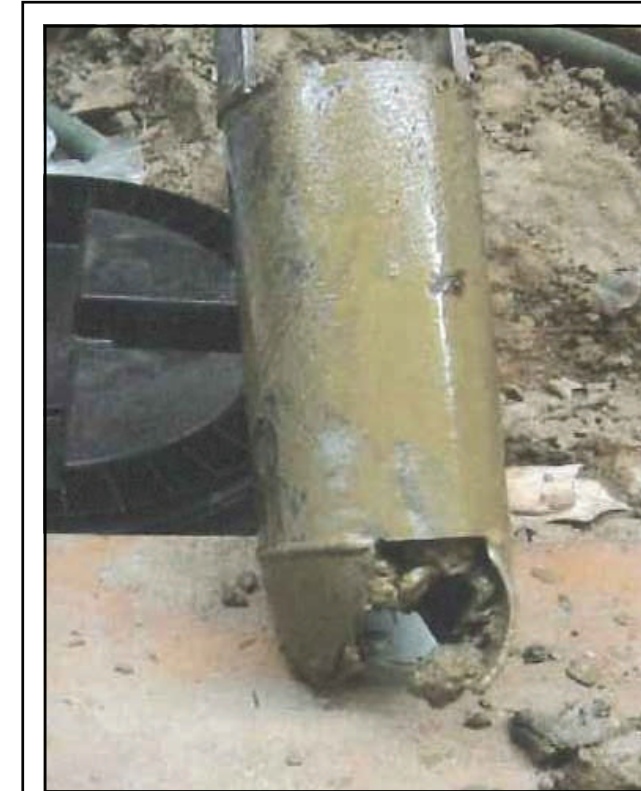
This photo depicts a soil sample collected from beneath a 550-gallon fuel oil UST that was closed in place at a commercial property. Closures in place require the laboratory analysis of soil samples and often require supplemental investigations.
