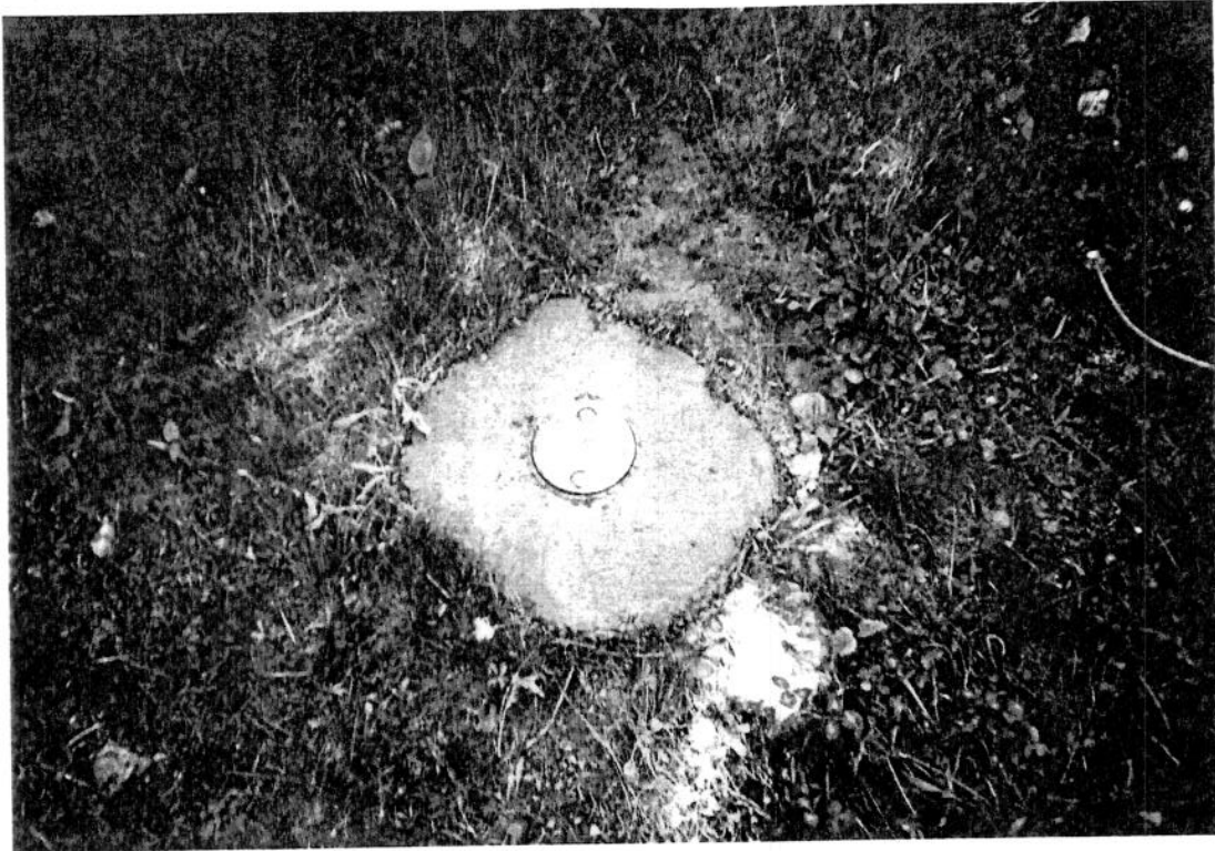
Monitoring Well WB-14 after repairs
