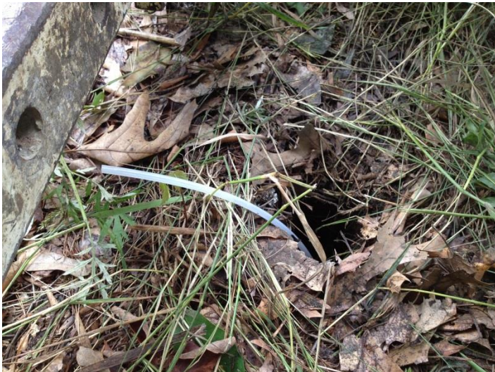
Photo 3 – Soil Gas Probe Prior to Finishing with a Roadbox
