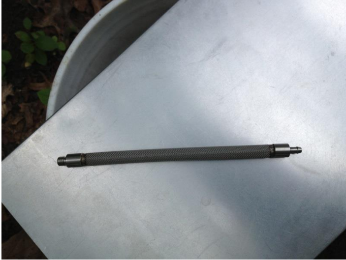
Photo 1 – Soil Gas Stainless Steel Vapor Sampling Tip
