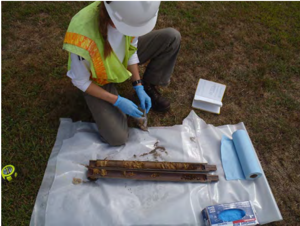
Photograph No. 40 A two-foot split spoon soil sample from SB-2.
