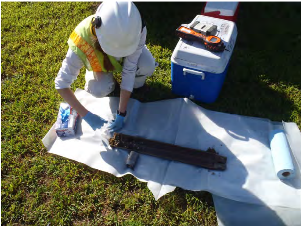
Photograph No. 38 Collection of a soil sample from a split spoon.
