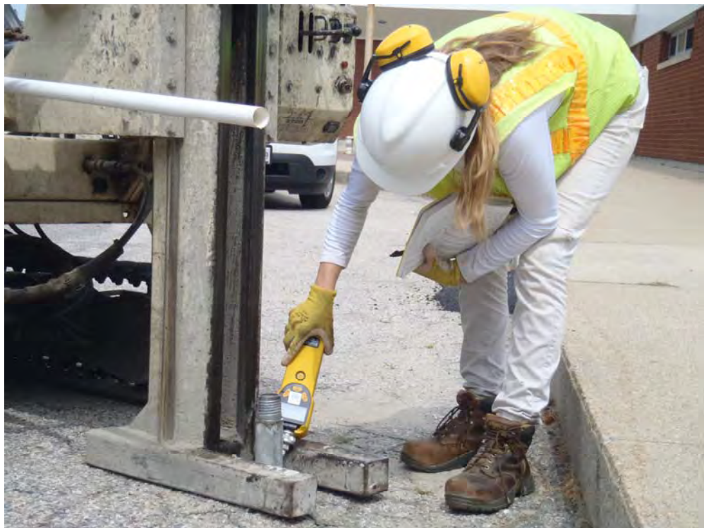
Photograph No. 32 Monitoring drilling atmosphere for VOCs during soil vapor point installation.
