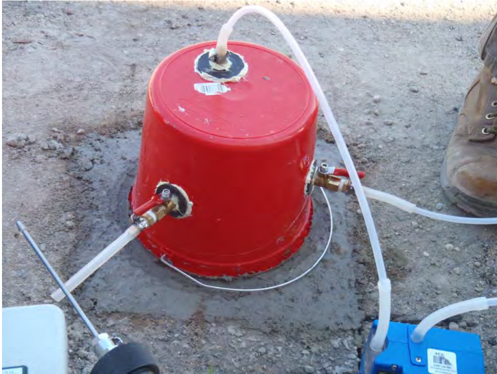
Photograph No. 36 Shroud for conducting a leak test on soil vapor points.
