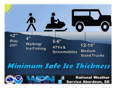
in reference to the ice quality. When ice undergoes patterns of freeze, thaw, and snow cover, the result is called white ice which has less structural stability than hard, black ice. Certain areas such as river outlets and springs will not freeze consistently with surrounding ice and may only be covered by unsafe skim ice. In safe practice, using an ice chisel or auger to test ice thickness in the areas you are walking and fishing can prevent accidents.
