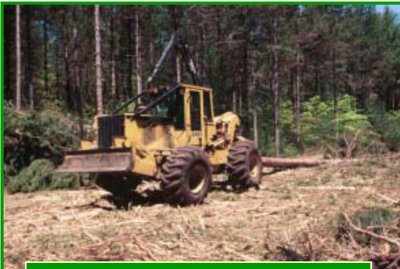
A skidder hauling a tree. Once the tree reaches the landing it will be bucked (cut to length) and then hauled to the mill.
