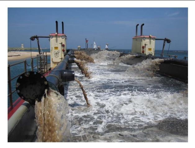
View from the deck of the CURRITUCK during the dredging of the Great Salt Pond Federal Navigation Channel, Block Island (RI) on June 1, 2010 (picture by Eric Schneider, DFW). The CURRITUCK is a special government owned (U.S. Army Corps. of Engineers) small hopper vessel with a split-haul and two hydraulic dredges.
