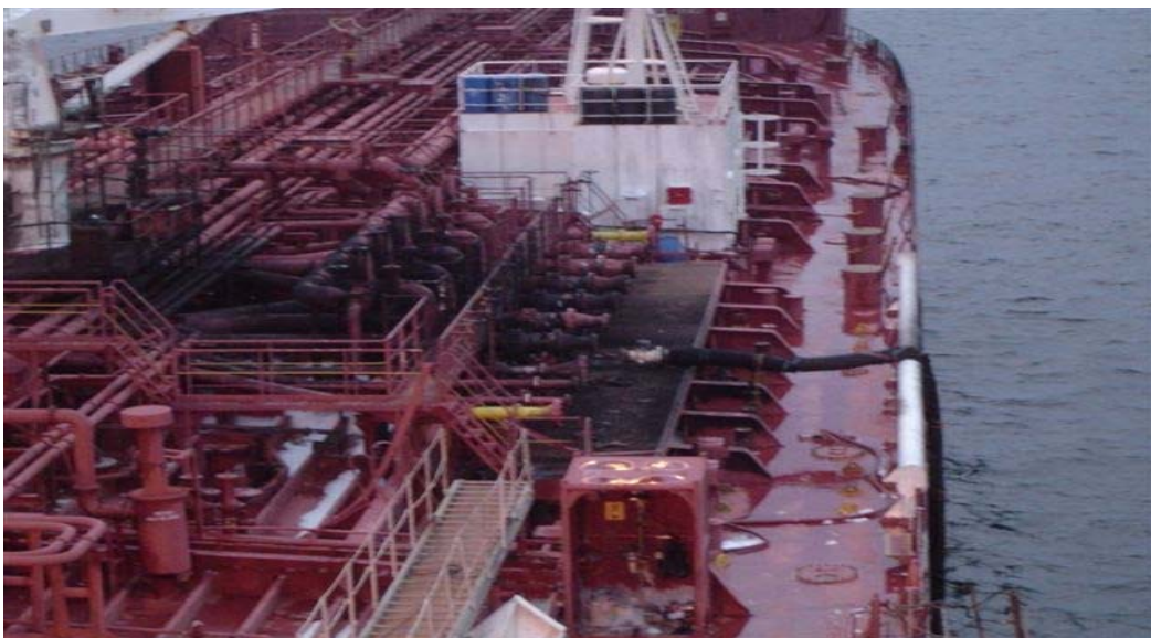
Figure 10. Fire Damage to deck of Nordeuropa , Motiva transfer hose remains attached to vessel.
