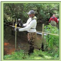
Robert Bradley from the USGS New England Water Science Center makes a streamflow measurement, an important piece of data in the stream gage network. Photo credit: USGS/Dennis LeBlanc.
