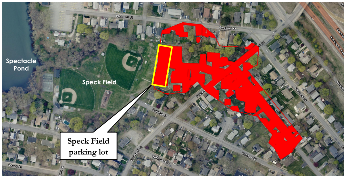
Figure 1: Speck Field parking lot catchment delineation (red outline) and impervious areas within the catchment (red fill).
