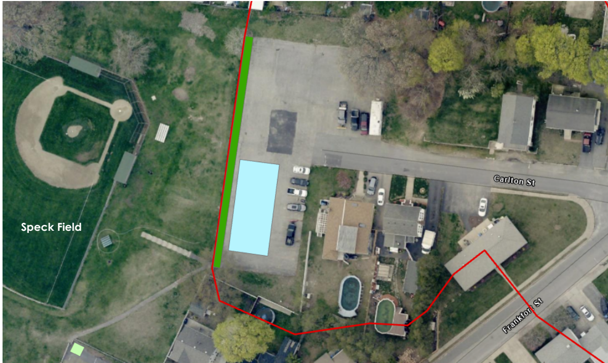
Figure 2: Conceptual layout of stormwater BMPs at the Speck Field parking lot. A bioretention swale is shown in green at the west edge of the parking lot, while the footprint of the underground infiltration practice is shown in blue.
