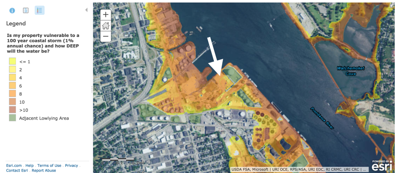
Figure 1. STORMTOOLS map, developed by RI Coastal Resources Management Council and University of Rhode Island, showing the depth of water during a 100 year coastal storm.
