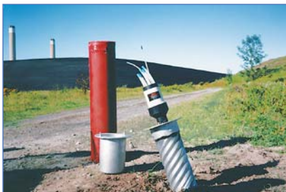
An investigation of hydraulic properties beneath a large waste site. Waterloo Multilevel Systems were chosen to allow water quality sampling and to help determine the zones of highest permeability within the aquifer.
