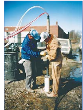
Detailed investigation of PCE delineation in carbonate bedrock. A cost analysis of the 14 Waterloo Systems compared with nested piezometers indicated savings both on the capital costs and on the on-going monitoring.
