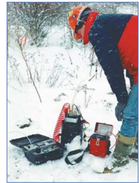
750ft. (230m) Waterloo System installation for a deep tunnel assessment study. Three zones monitored with dedicated Double-Valve Pumps and pressure transducers. Picture shows technician obtaining pressure measurements and groundwater samples with portable readout and pump control unit.
