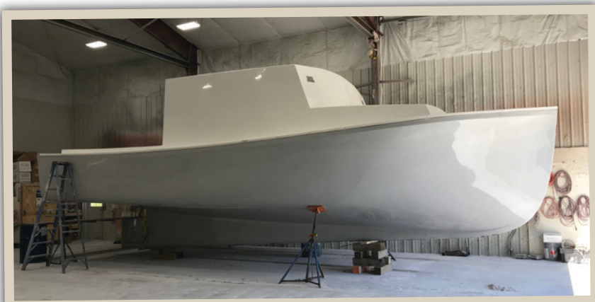
The hull out of the mold and in place during the early part of the build at SW Boatworks in Lamoine, ME in 2019.
