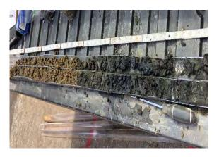
**Photo 6:** SB-4 from 10'-15' bgs. Fine to coarse sand with gray silt and little sand at depth.
