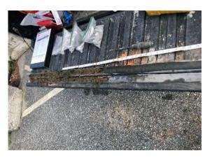
**Photo 14:** SB-10 from 10'-15' bgs. Fine to coarse sand and gray clayey silt with trace gravel
