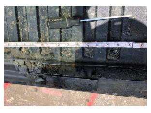
**Photo 8:** SB-5 from 5'-10'. Fine to coarse sand and trace silt. Gravel at 5' depth.
