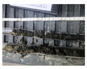
**Photo 3:** SB-3 from 5'-10' bgs. Fine to coarse sand with trace silt and few brick fragments.
