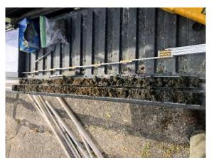
**Photo 12:** SB-9 from 5-10' bgs. Fine to coarse sand and trace silt and clay.
