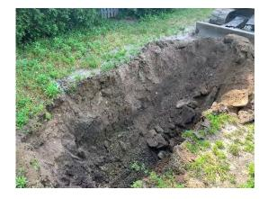
**Photo 20:** TP-8 Fill observed from 0' to 3' bgs.
