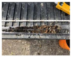
**Photo 11:** SB-9 from 0'-5' bgs. Fill with asphalt, sand with little silt. Trace shells, ash, and glass.
