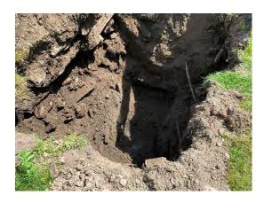
**Photo 19:** TP-6 Fill observed from 0' to 8.5' bgs.
