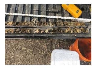
**Photo 15:** SB-11 from 0'-5' bgs. Fill with asphalt, fine to coarse sand, trace silt and cobbles.
