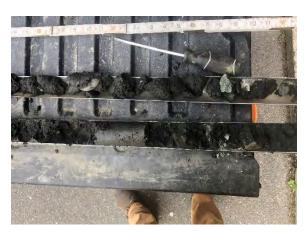
**Photo 4:** SB-3 from 10'-15' bgs. Gray fine to coarse sand and hardpacked silt at depth.
