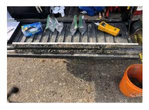
**Photo 16:** SB-11 from 10'-15' bgs. Alternating sand and clayey silt.
