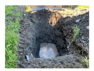
**Photo 17:** TP-1 Fill observed from 0' to 3' bgs.
