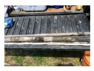
**Photo 9:** SB-8 from 0-5' bgs. Fill with asphalt, sand, crushed stone and trace silt and gravel.
