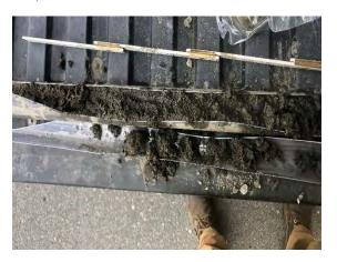
**Photo 2:** SB-2 from 10'-15' bgs. Gray hardpacked sand and trace silt and clay.
