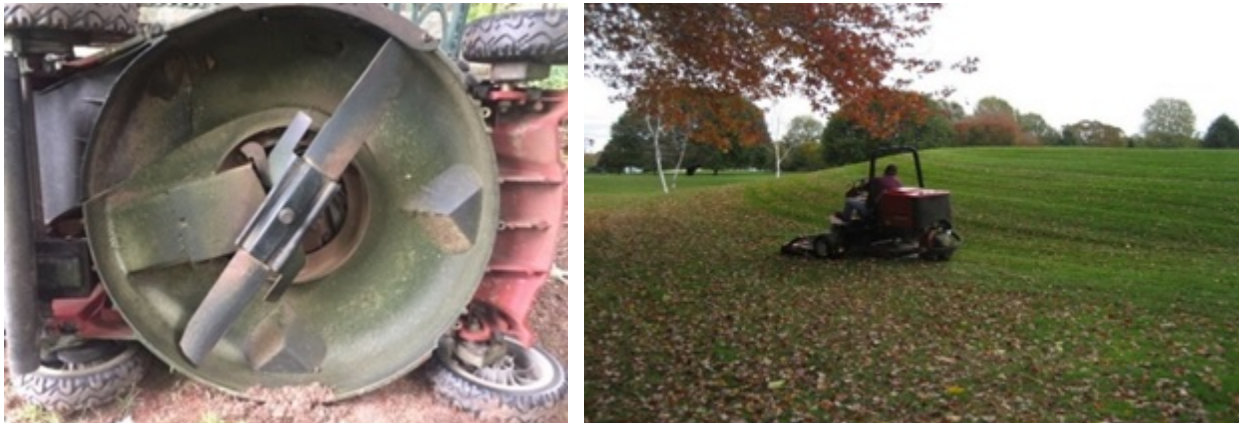
Figure 6-4. Rotary mowers are used for rough and surrounds (bunker, green, and tee). Sharp rotary blades are necessary for a quality cut and plant health.
