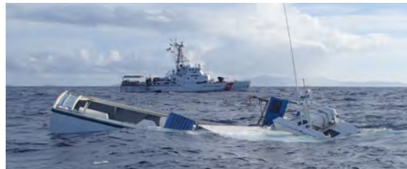
Figures 22–24: Flooding of the Sea Shepherd from damage due to the collision. The vessel sank about 2 hours after it was struck.
