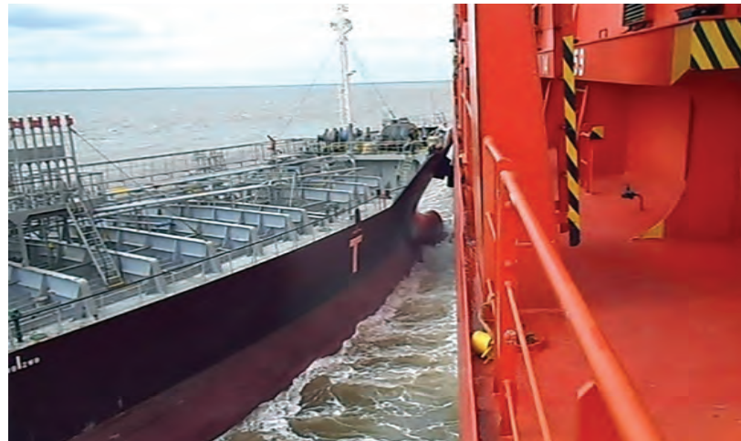
Figure 13: Video screen capture of tanker Chembulk Houston's bow and anchor in contact with containership Monte Alegre .
