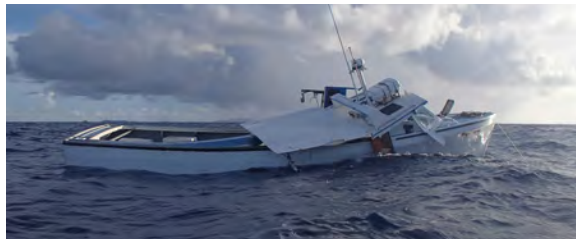
Figures 22–24: Flooding of the Sea Shepherd from damage due to the collision. The vessel sank about 2 hours after it was struck.
