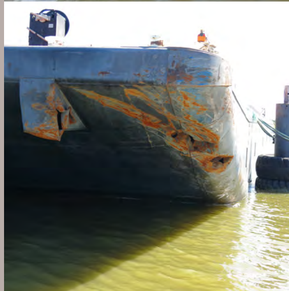
Figure 10: Damage to the bow of barge Kirby 29116 resulting from the collision.
