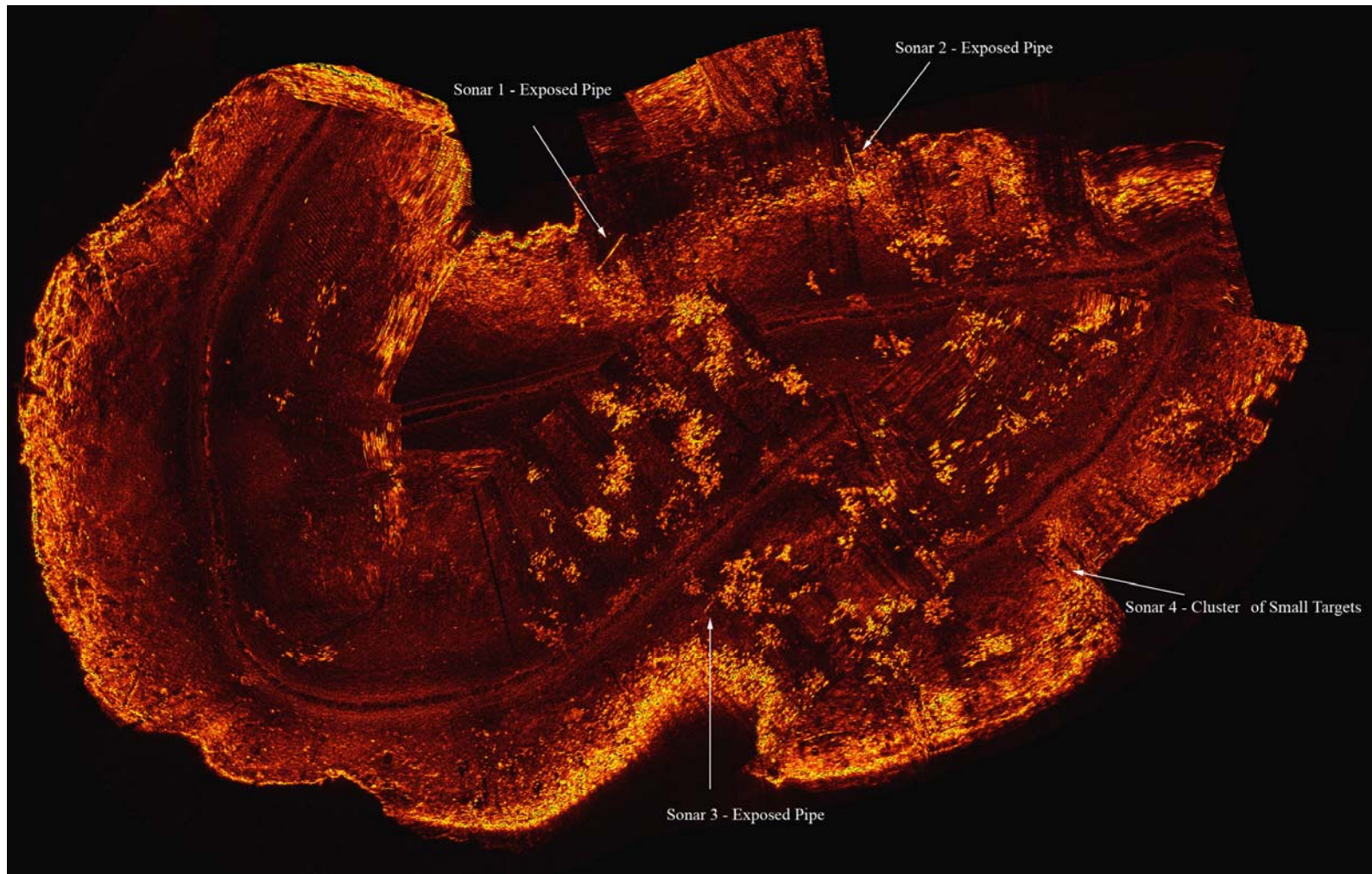
Figure 5. Side scan sonar mosaic with sonar targets indicated. Light patches in the cove are clusters of aquatic vegetation. Fallen trees and debris can be seen along the shorelines.
