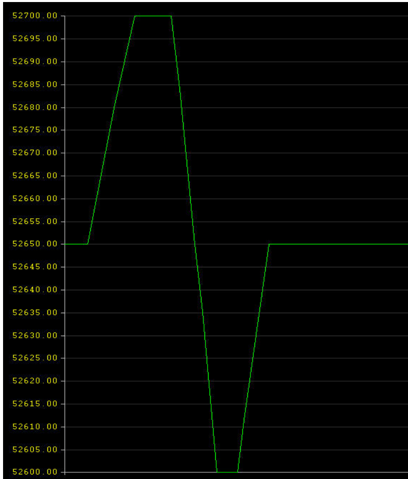
Figure 3. Magnetic signature of 100 gamma drum target.
