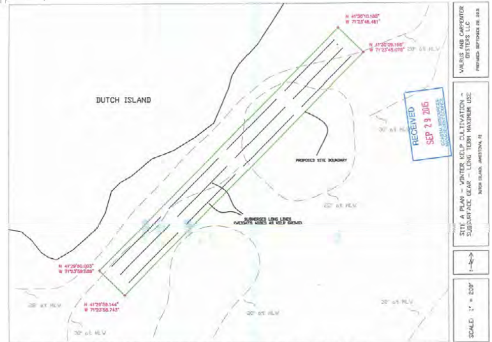
Figure 10: Plan view of site A with maximum winter use for kelp cultivation (gear below water surface displayed)
