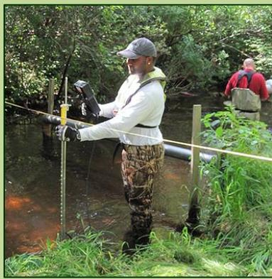
*Robert Bradley from the USGS New England Water Science Center makes a streamflow measurement, an important piece of data in the stream gage network. Photo credit: USGS/Dennis LeBlanc.*
