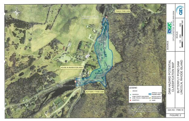
Dam failure inundation map for Butterfly Pond Dam (No. 097), Lincoln. A map specific to each dam is included in the EAP for that dam.
