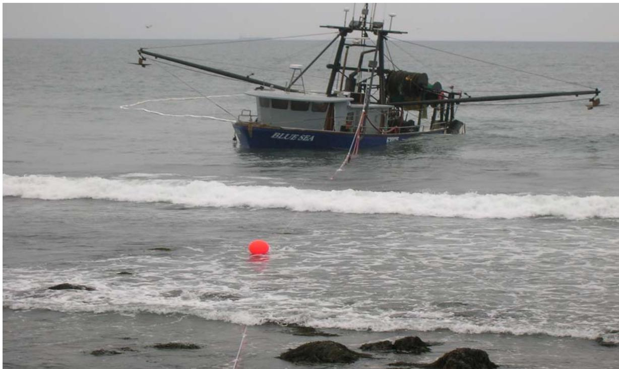
Figure 7. F/V Blue Sea with support line and transfer hose.
