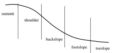
**Slope** - You will be required to record the slope of the land where the pit has been excavated. A clinometer will be available at each pit for determination of slope.
