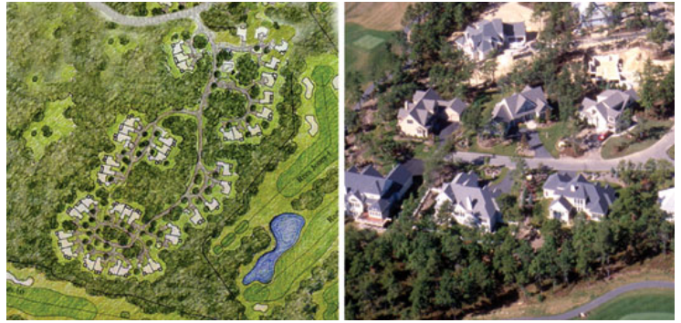
Low impact cluster design subdivision. (Source: Massachusetts Executive Office of Energy and Environmental Affairs)
