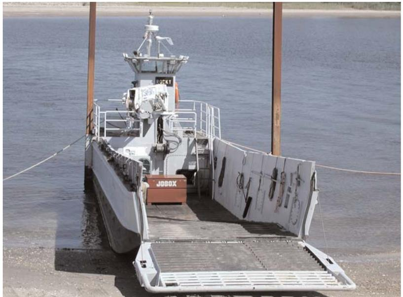
A specially equipped 58-foot mechanized landing craft uses an on-board crane to access large debris on the shoreline or in the water.
