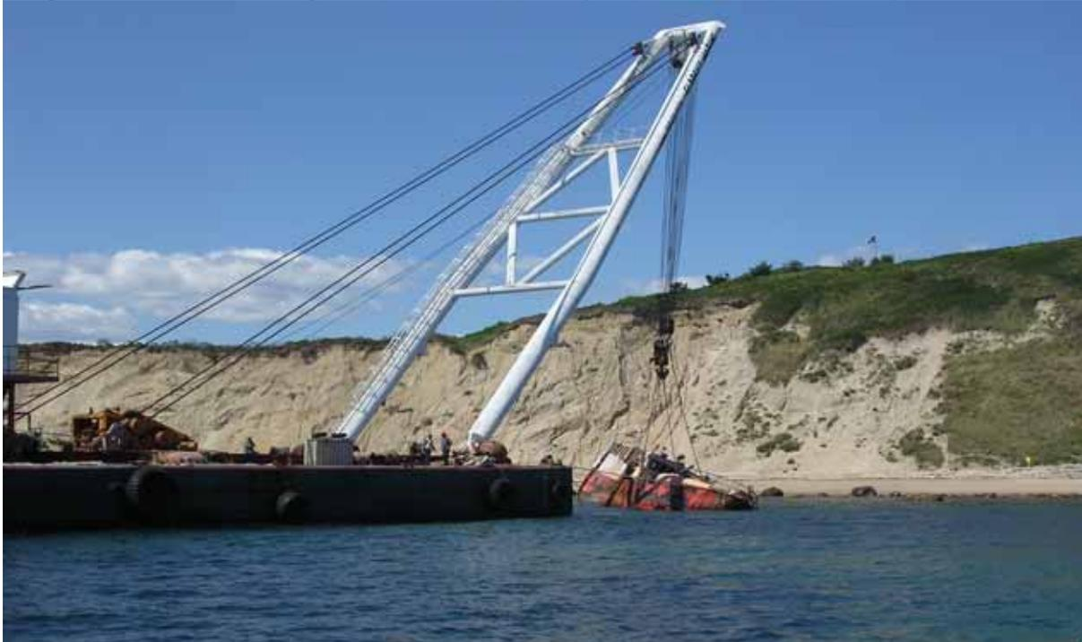
Figure 5. Crane Barge OVUS I Prepares to Lift Bow Section
