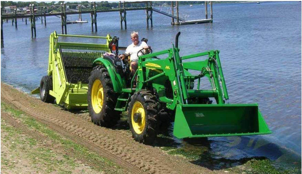
Figure 9. Barber Surf Rake Collecting Sea Lettuce along Conimicut Shore
