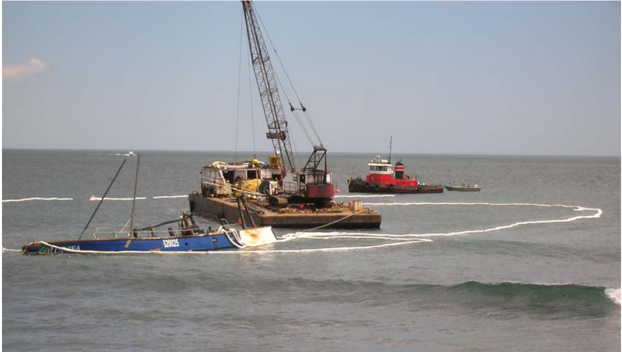
Figure11. F/V Blue Sea and barge in containment boom.
