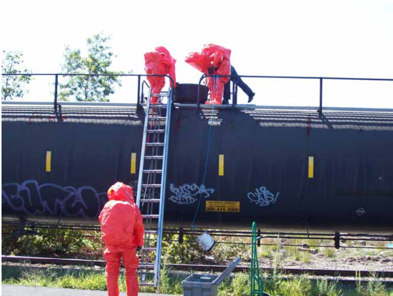
Figure 6 RI and CT HazMat Teams applying a patch kit to stop a notional leak
