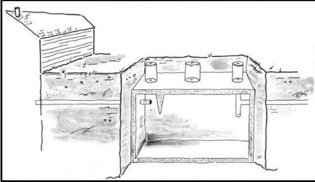
**Figure 1.3a** Cut-away view of a conventional 1000-gallon septic tank. Wastewater flows by gravity from the building sewer to the septic tank, followed by the distribution box and then to the soil absorption system.
