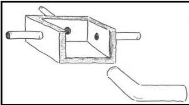
**Figure 1.3b** Exploded diagram of a conventional distribution box.
