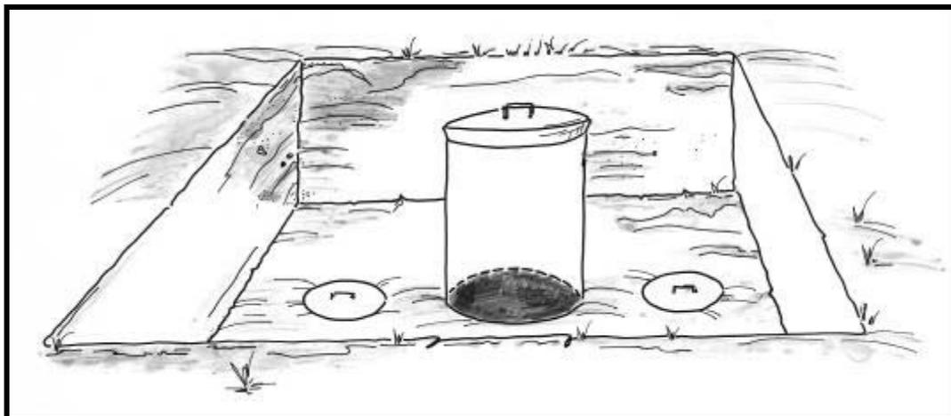
**Figure 4.3c** Improper installation of well ring risers with the septic tank main access (manhole) cover moved to the top of the well ring. This provides a poor fit, which may result in leakage as well as chipping of the concrete.
