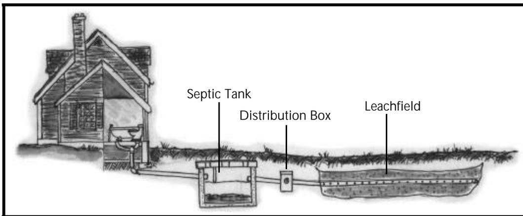
Figure 5.1 Diagram of a conventional septic system
