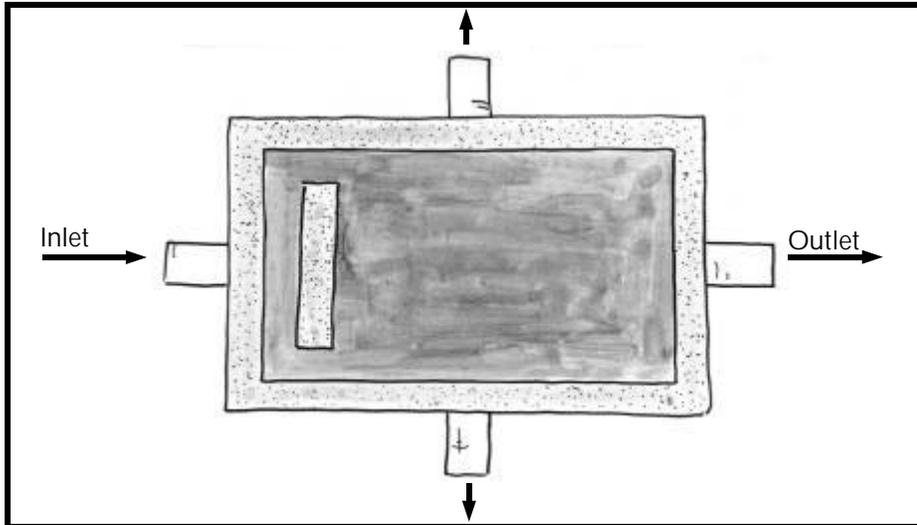
Figure 4.1 Top view of a distribution box
