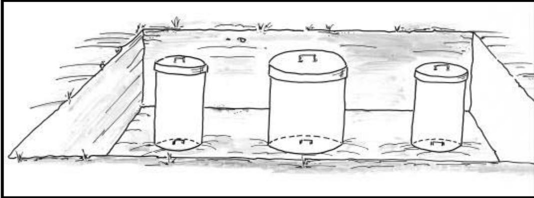
**Figure 4.3b** Proper installation of concrete well ring risers on the main access (manhole). Main access (manhole) cover remains on the tank; well rings are capped with a concrete cover that overlaps the outside of the rings to prevent leakage.
