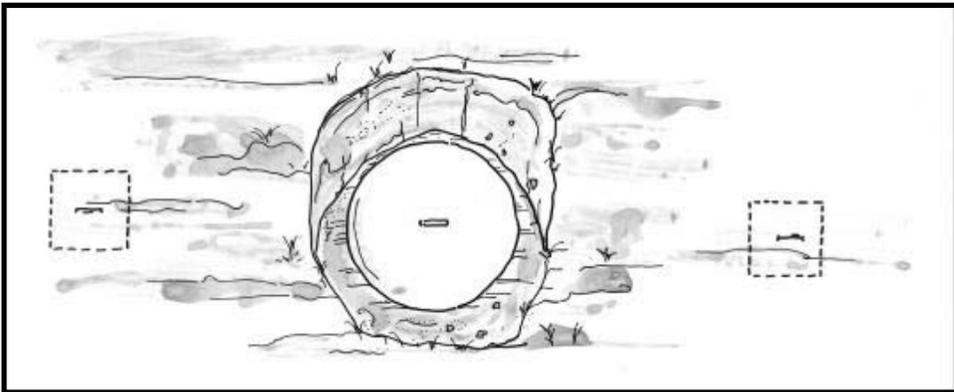
**Figure 4.2b** Top view of a typical unearthed septic tank main access (manhole). (Current regulations require a manhole and two inspection ports. DEM is revising the regulations to require two 20-inch manholes at the influent and effluent ends of the tank and no center manhole.)
