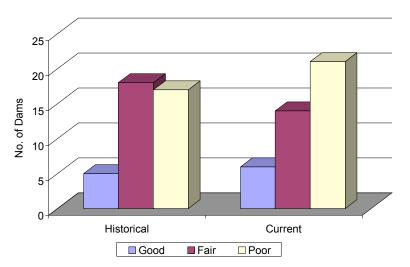
The charts illustrate general trends of improving conditions of the high hazard dams and deteriorating conditions for the significant hazard dams. Many of these significant hazard dams will likely be reclassified as either low or high hazard dams through DEM's ongoing classification assessment.
